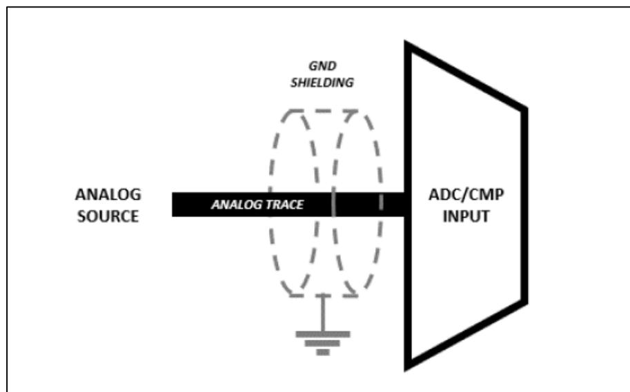
图 5-1 Shielding of analog signals
