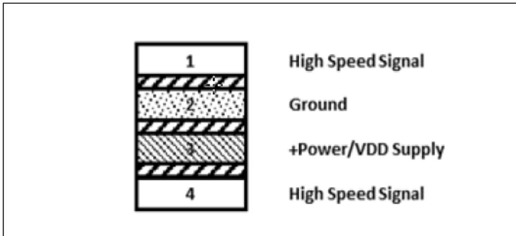
图 11-5 Recommended PCB layer stack-up
